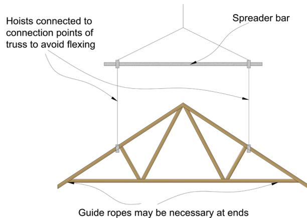
Figure 6: Mechanical lifting
