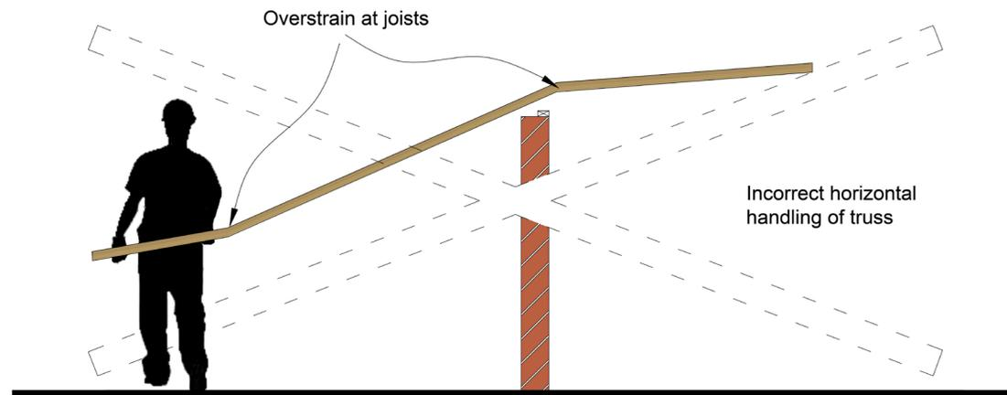
Figure 5: Avoid bending or see-sawing of trusses
