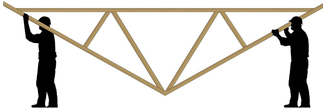
Figure 4: Suggested method of manual lifting
