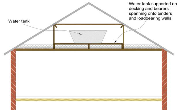
Figure 9: Tank stand configuration
