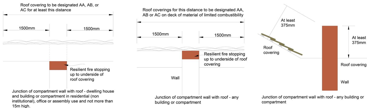
Figure 13: Typical fire stopping details
