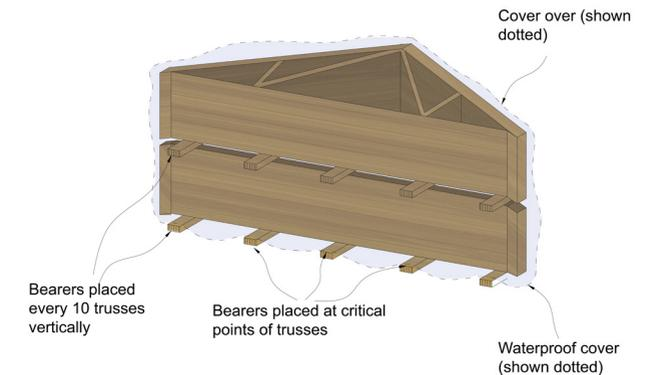
Figure 3: Horizontal storage of trusses
